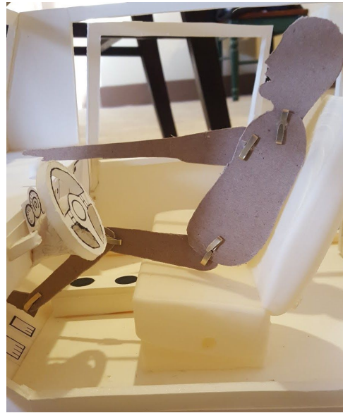
Side View- showing how 95th Percentile male fits in the Vehicle
